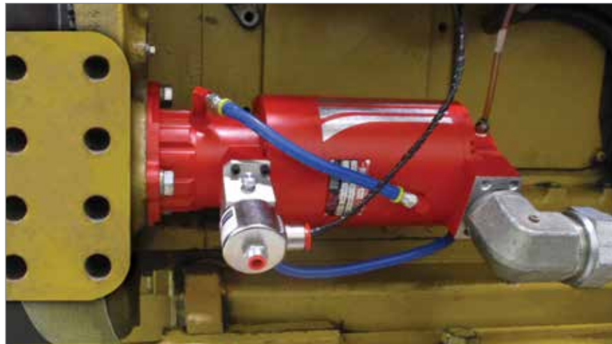
Single TurboTwister T6C on CAT 3516
