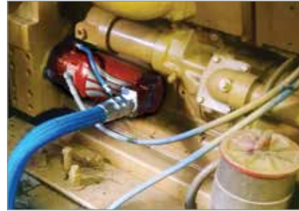
T6C TurboTwister on Caterpillar 3516
