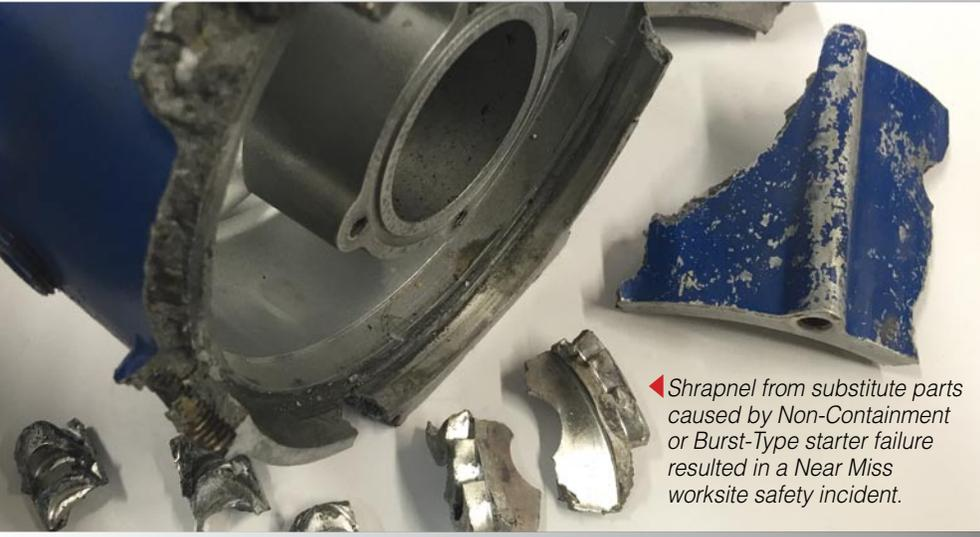
◀ Shrapnel from substitute parts caused by Non-Containment or Burst-Type starter failure resulted in a Near Miss worksite safety incident.
